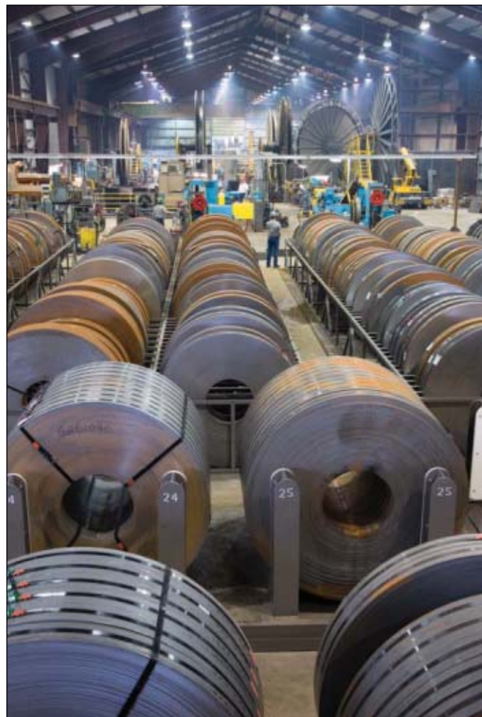
Coiled strip stock stands ready for forming and welding at Tenaris Coiled Tubes' downhole manufacturing facility in Houston (Fig. 1; photo from Tenaris).
